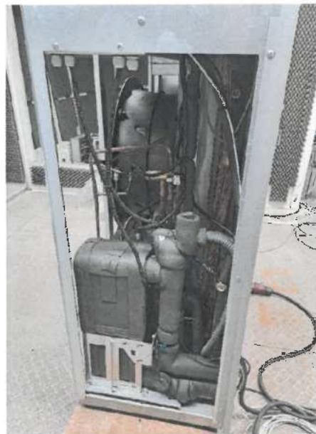
Heat pump AirAdapt 4-20 - outdoor unit – Without cover –
