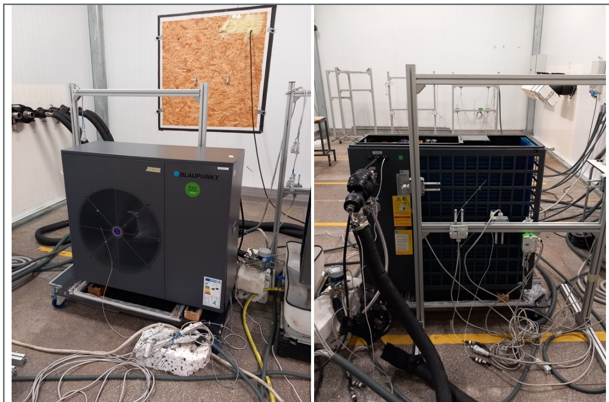
Figure 1. Installation of the test sample.
