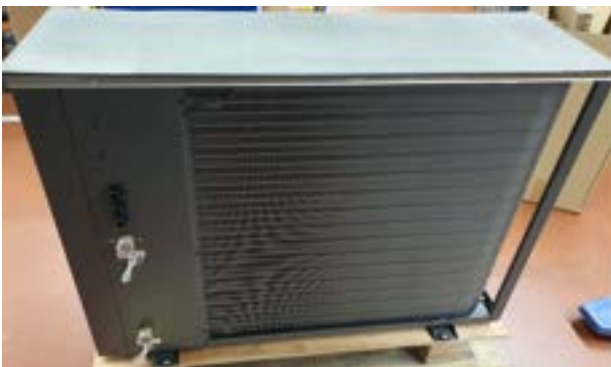
Verdampfer (Evaporator)
