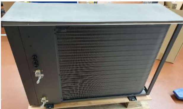
Verdampfer (Evaporator)
